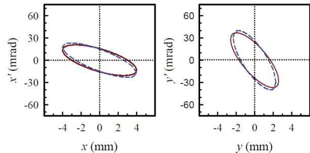
Figure 5: Phase ellipses in the  $x$  and  $y$  planes for matching at the inflector entrance with average current  $I = 5$  mA.
