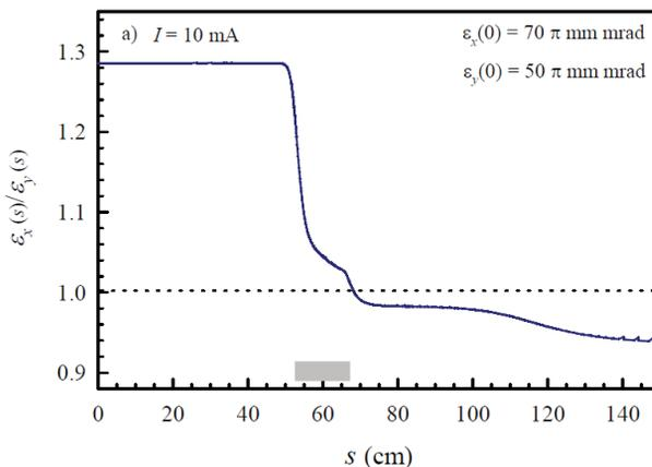
Figure 4: Evolutions of transverse projected emittances obtained at  $I = 10$  mA for non-axisymmetric input beam.
