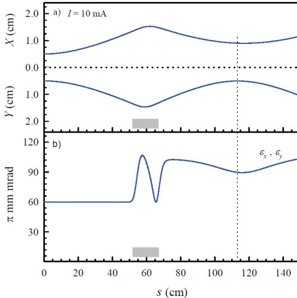
Figure 3: Evolution of (a) beam envelopes and (b) projected emittances for  $I = 10$  mA at 80 keV proton.
