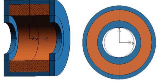
Figure 1: Half 3D model and entrance pole face of the elliptical solenoid.
