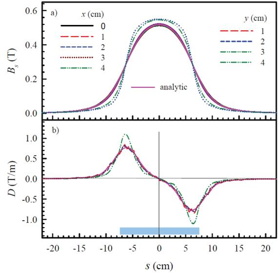
Figure 2: Plots of axial magnetic field  $B_s$  and parameter  $D$  as a function of  $s$  at different values of  $x$  and  $y$ .
