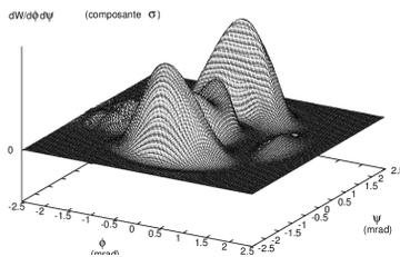
Figure 7: Interferential "Newton rings" from 1 TeV proton radiation. Two light sources interfere in this pattern: dipole edge and undulator, distant 1 m.
