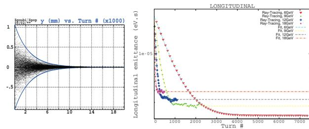
Figure 5: Left: damping of vertical motion to quasi-zero (no scattering) over a few damping times, uncoupled lattice, 6 GeV. Right: damping of the longitudinal emittance, numerical data are fitted with  $\epsilon(t) = \epsilon_0 e^{-t/\tau} + \epsilon_f (1 - e^{-t/\tau})$ , for 6, 9, 12 and 18 GeV.
