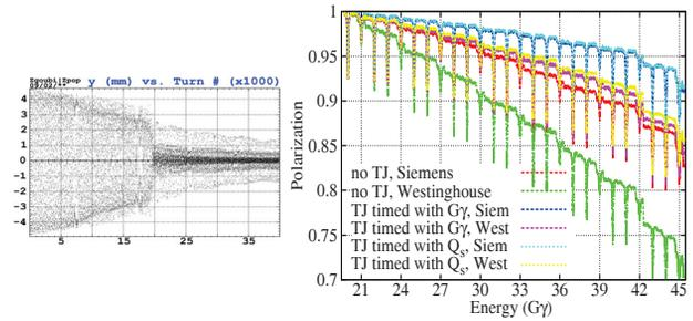
Figure 3: Left: horizontal excursion from injection to transition energy, 5 particles launched at 72 deg. betatron phase intervals on  $\epsilon_x = \epsilon_y = 2.5\pi$  mm.mrd invariants, showing coupling and betatron resonance effects induced by the snakes. Right: polarization vs. energy depending on AGS jump quad timings and main magnet power supply used,  $10^3$  particles in a realistic 6-D bunch.
