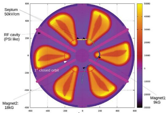
Figure 6: A design of the injection line into a molecular  $H_2$  separated sector cyclotron.
