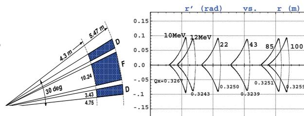
Figure 8: 150 MeV radial triplet FFAG, horizontal dynamic aperture and corresponding tunes at various energies. Not shown here: Zgoubi's semi-analytical FFAG triplet magnet model and the OPERA field maps give similar results [25].
