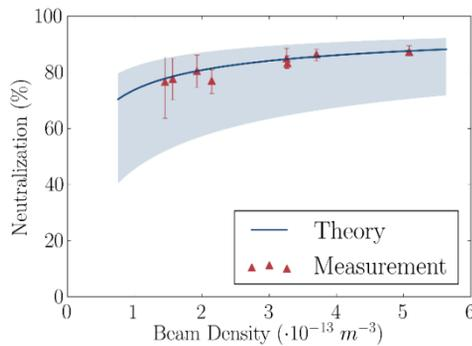
Figure 4: Neutralization factors of a proton beam for different beam densities in the LEBT of the LEDA injector source. The solid line indicates the model prediction and the shaded area the uncertainty due to the not well known cross sections and uncertainties in the pressure measurement.
