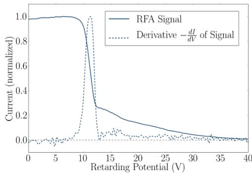
Figure 2: Typical RFA spectrum obtained with SuSI (solid line) and the first derivative (dashed line) which corresponds to the secondary ion energy distribution.
