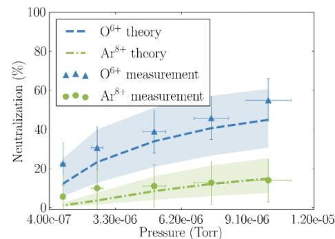
Figure 5: Neutralization factors of a 200 eμA Ar<sup>8+</sup> and a 700 eμA O<sup>6+</sup> beam at different vacuum pressures in the LEBT of the SuSI source at NSCL. The dashed lines indicate the model description with the shaded areas being the uncertainty due to the not well known cross sections.
