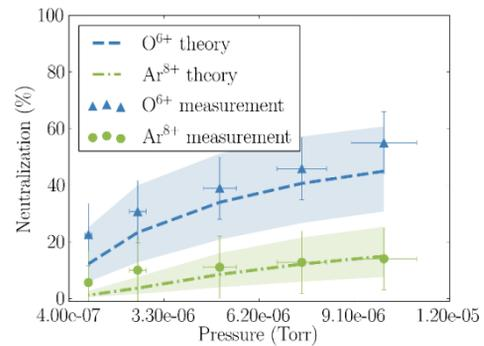
Figure 5: Neutralization factors of a 200 eμA  $Ar^{8+}$  and a 700 eμA  $O^{6+}$  beam at different vacuum pressures in the LEBT of the SuSI source at NSCL. The dashed lines indicate the model description with the shaded areas being the uncertainty due to the not well known cross sections.
