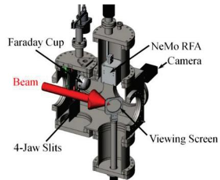
Figure 3: Diagnostic box in the SuSI LEBT with RFA and beam imaging devices.
