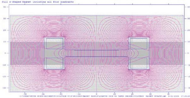
Figure 2: POISSON Superfish simulation of magnetic field in the iron electromagnet yoke.
