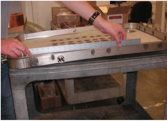
Figure 6: Warping of the vacuum chamber due to mechanical stresses after welding.
