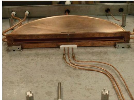
Figure 8: Front view of the dee, showing the placement of the ion source.
