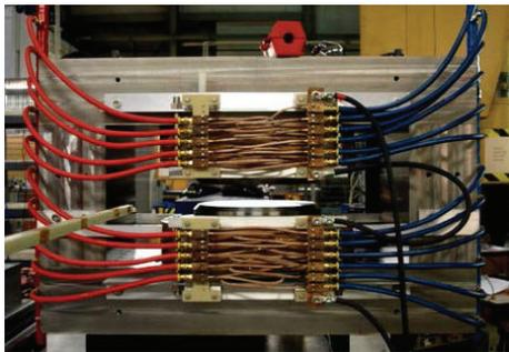
Figure 3: Completed electromagnet with water distribution manifold.
