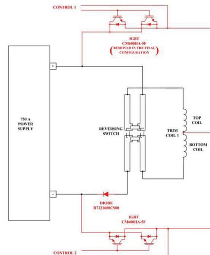
Figure 1: Trim coil unbalance circuitry. The original trim coil system is displayed in black and the modifications are in red. Two parallel IGBT transistors are connected across each coil. The top IGBT transistors connected to the positive output are removed in the final configuration. A power diode is also added in the final configuration between the power supply negative output and the reversing switch, allowing to shunt half of the trim coil current.
