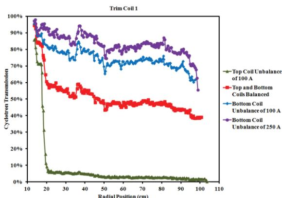
Figure 2: Dee probe measurements of 266 MeV  $\text{Cr}^{+14}$  ion beam. The red line with square markers shows trim coil 1 driven by 500 A in balanced configuration. The green line with triangle markers shows 100 A unbalance, shunting current around the top coil. The blue line with diamond markers shows 100 A unbalance, shunting current around the bottom coil. The violet line with circle markers shows 250 A unbalance of the bottom coil.
