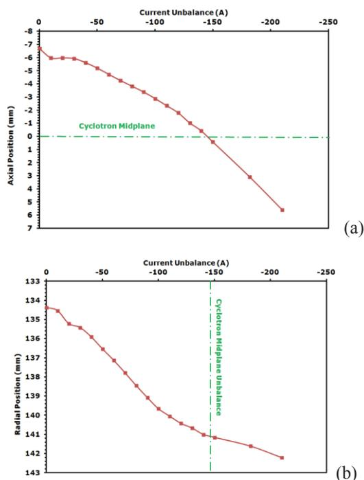
Figure 3: Center of mass position versus current unbalance (a) Axial position. (b) Radial position.
