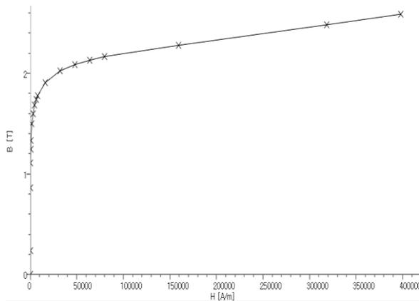
Figure 2: B-H curve of magnet material.
