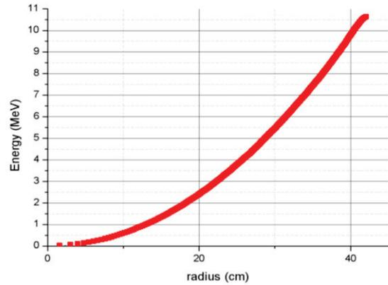
Figure 4: Energy of orbit as a function of radius.
