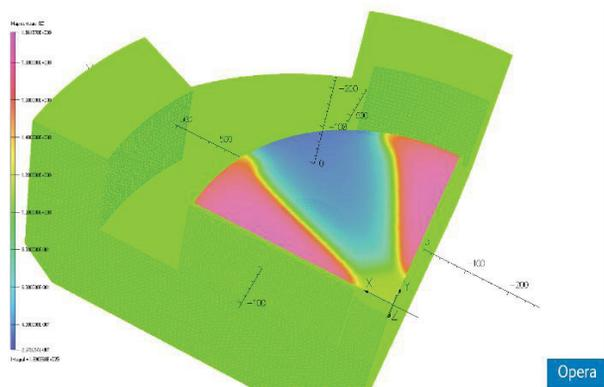
Figure 3: Magnetic field distribution in magnet pole.
