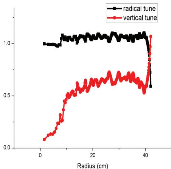
Figure 7: Tunes as a function of radius.
