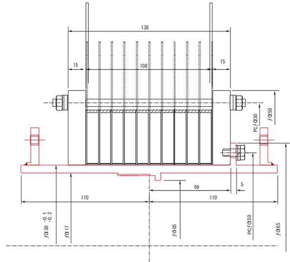
Figure 3: A cross sectional structure of the upper half of the cylindrical magnet. Each double pancake is sandwiched by 1 mm thick cooling plates made of copper.
