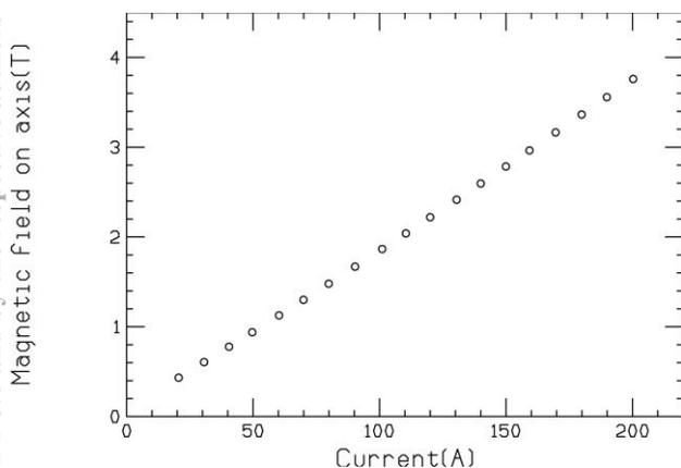
Figure 6: Excitation results of the fabricated magnet.
