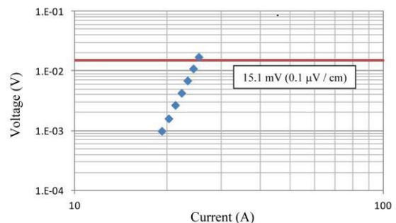
Figure 4: Results of  $I_c$  measurement at 77 K. The total length of wire is 1530 m.
