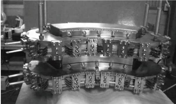
Figure 2: Assembled 3 T dipole magnet.
