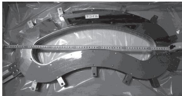
Figure1: Lower coil of the dipole magnet.
