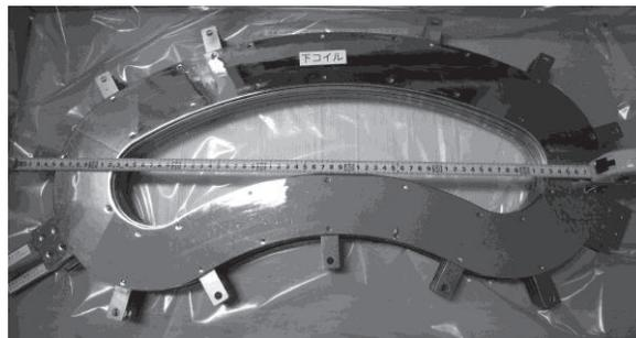
Figure1: Lower coil of the dipole magnet.
