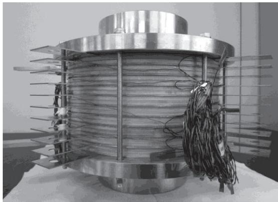
Figure 5: Stacked coils fixed to the bobbin.
