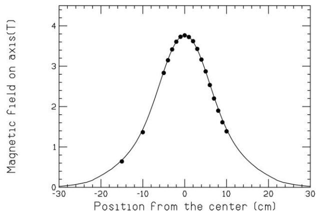
Figure 7: Field distribution along the axis. the solid line shows results of the numerical simulation by TOSCA.
