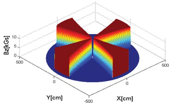
Figure 4: Field map for the 100 MeV Injector cyclotron.
