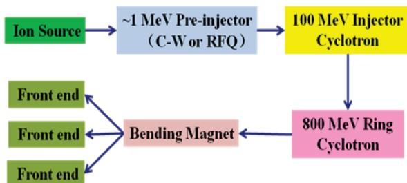
Figure 1: The block diagram of the BRIF-III proposal.
