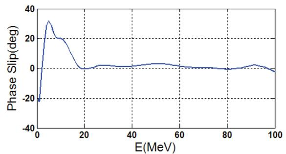
Figure 5: Phase slip of the 100 MeV injector cyclotron with the energy gain per-turn of 2 MeV.
