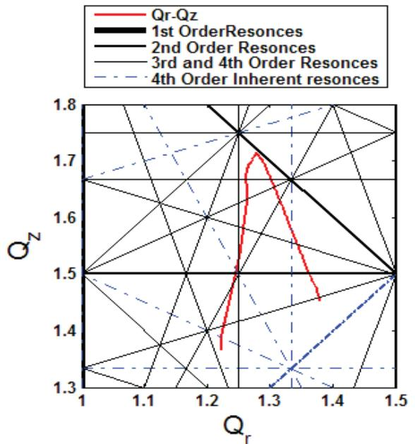
Figure 6: Tune diagram for the 100 MeV injector cyclotron.
