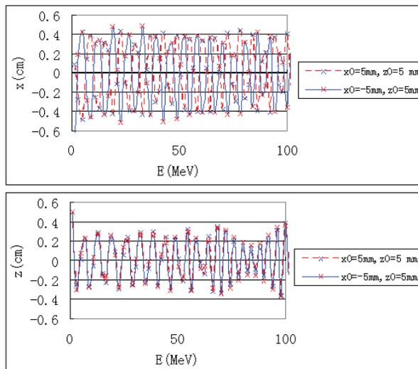
Figure 7: The radial (up) and vertical (down) oscillations of two off-centered particles.
