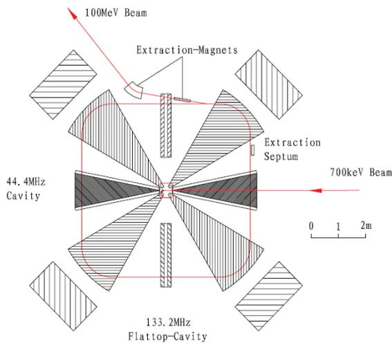
Figure 3: Layout sketch of the 100 MeV injector cyclotron.
