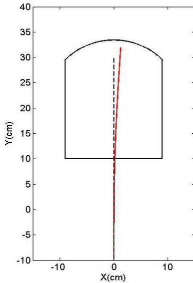
Figure 5: Beam trajectory through the magnet.
