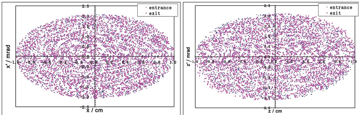
Figure 6: Phase distribution at the entrance and exit of the magnet.
