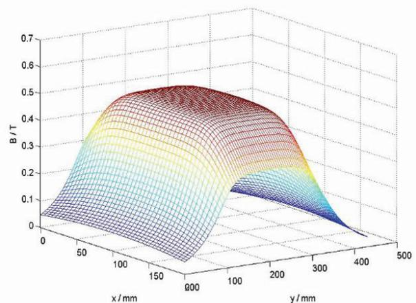
Figure 4: Measurement of combination magnet and the field distribution on the mid-plane.
