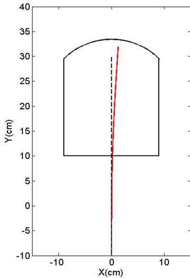
Figure 5: Beam trajectory through the magnet.
