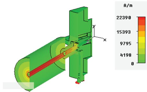
Figure 5: Surface current distribution 60MeV.
