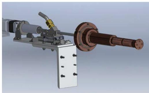
Figure 10: Tuning mechanism.
