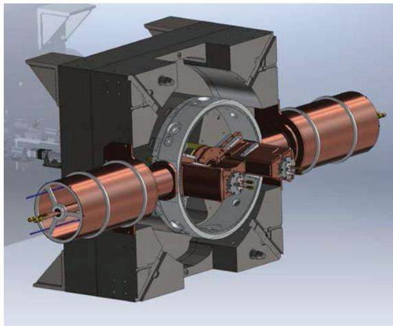
Figure 8: Resonators installed in magnet.
