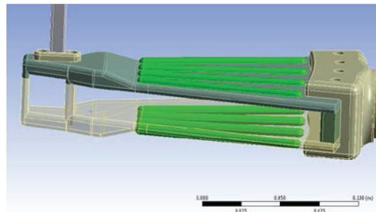
Figure 6: Dee plates with heat pipes (green).
