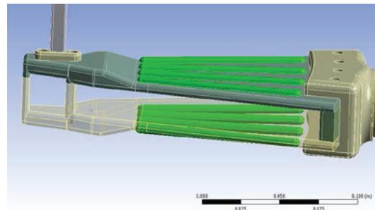
Figure 6: Dee plates with heat pipes (green).
