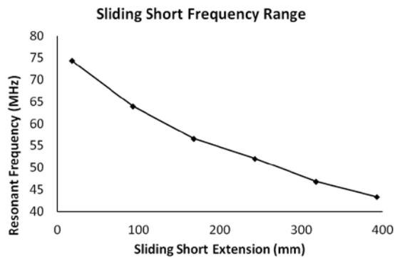
Figure 3: Frequency versus sliding short extension.
