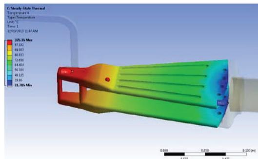
Figure 7: Dee temperature profile for hottest case, min 32°C and max 105°C.
