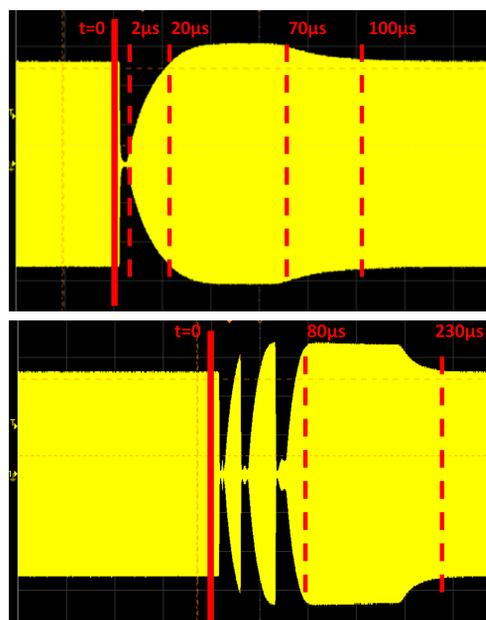
Figure 3: Cavity voltage during the detection and recovery from a single spark (top) and triple spark (bottom).
