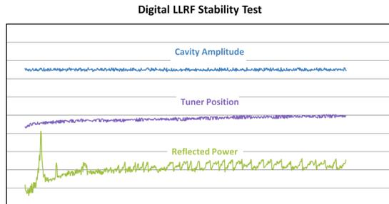
Figure 4: Initial one-hour stability test on a single resonator cyclotron (vertical axes are unscaled).
