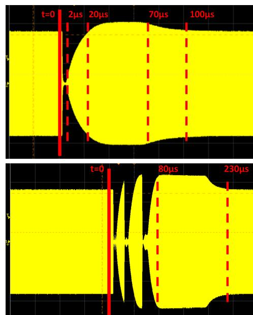
Figure 3: Cavity voltage during the detection and recovery from a single spark (top) and triple spark (bottom).
