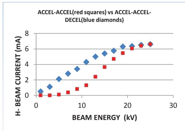
Figure 5: A comparison of the accel-accel and the accel-accel-decel electrode systems.
