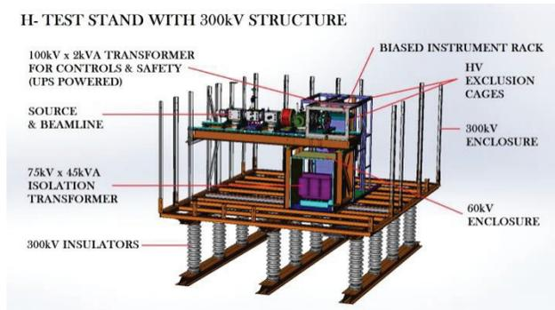
Figure 1: H<sup>-</sup> test stand with the 300 kV platform.
