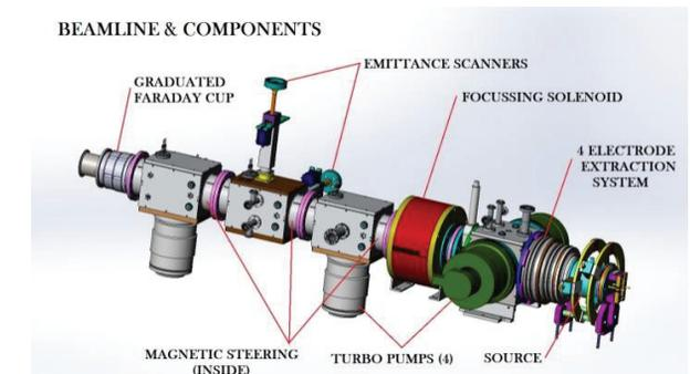
Figure 2: The beam line with the source, extraction system, diagnostics elements and the vacuum components.
