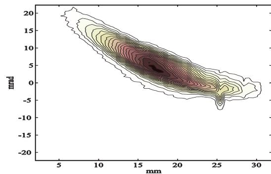
Figure 6: The emittance measurements were performed at 15 mA H<sup>-</sup> current at 25 kV. 90%, 86%, 63% and 39% found to be 44, 39, 29 and 20  $\pi$ -mm-mrad respectively
