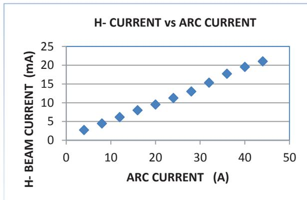
Figure 4: H<sup>-</sup> current vs arc current.
