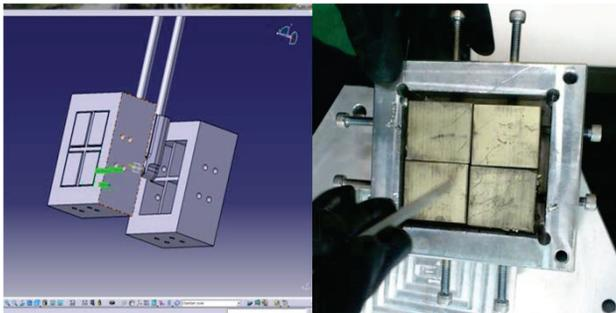
Figure 9: The four permanent magnet for distribution of magnetic field.
