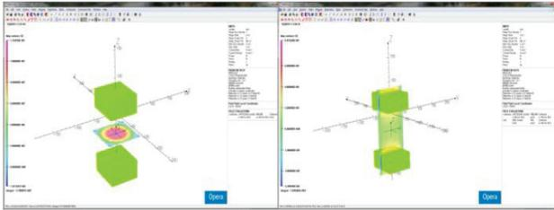
Figure 8: The magnetic field distribution in the PIG ion source.
