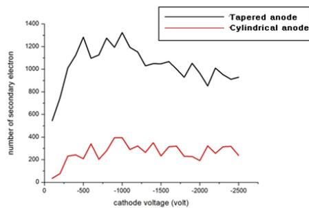
Figure 4: The number of secondary electron in two types of anode.
