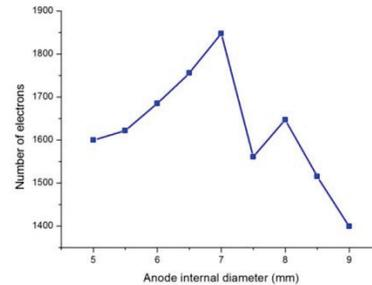
Figure 5: The number of secondary electron in tapered anode by varying diameter.
