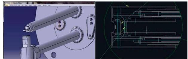
Figure 6: The design of PIG ion source.
