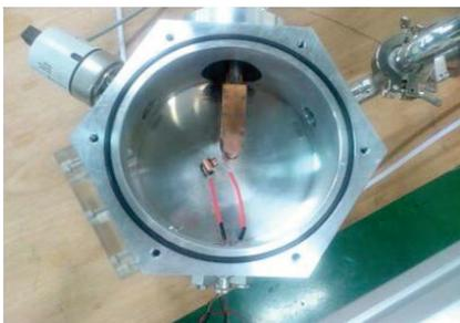
Figure 10: The vacuum chamber for testing PIG ion source.
