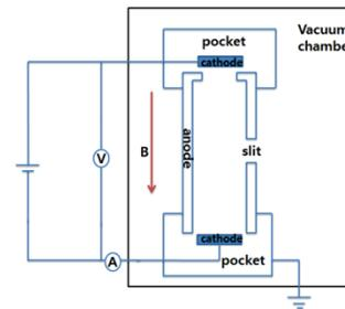
Figure 1: Schematic of the PIG ion source.
