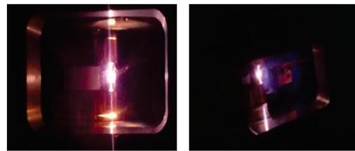
Figure 11: The plasma discharge in PIG ion source.
