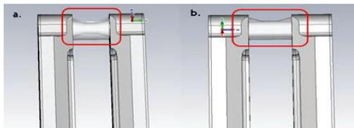
Figure 3: The optimization of anode shape.
