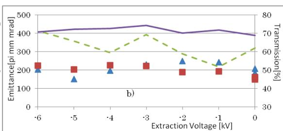
Figure 4: Squares are for x emittance measured by emittance monitor installed just after the FC3 and triangles are for y emittances. The dashed line shows the calculated emittance at the baffle slit the end of extraction system by IGUN code. The beam transmission between FC1 and FC3 is shown by solid line
