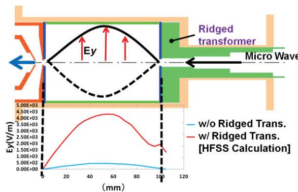
Figure 7: The result of micro wave inside plasma chamber calculated with ANSYS HFSS.
