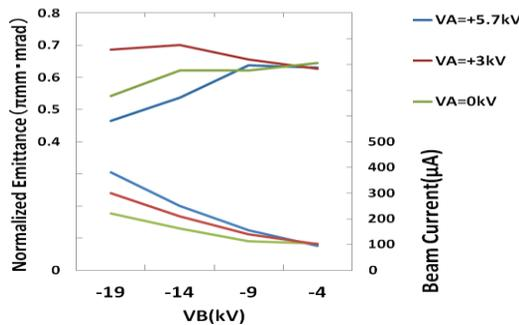
Figure 6: The proton beam production test with several conditions of applied extraction voltages. VA is the voltage of A-electrode shown in Figure 5. VB is for B-electrode. VC the C-electrode voltage is fixed to +4kV and VD is on ground. Upper lines show measured normalized emittances for each VA and VB. Lower lines show measured beam currents.
