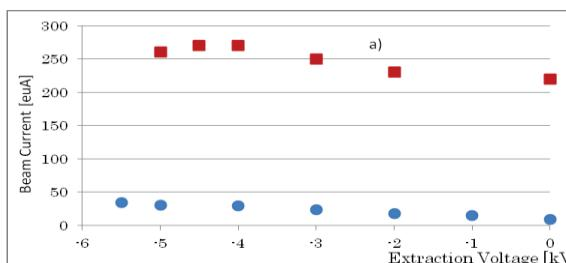
Figure 3: Beam currents versus extraction voltage. Circles show the current of 12C5+ made by CO<sub>2</sub> gas and squares show the 12C5+ by CH<sub>4</sub>.
