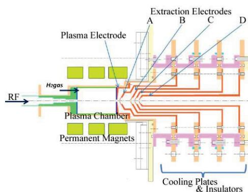
Figure 5: Schematic view of 2.45 GHz HIP-ECR. Extraction electrodes are connected to cooling plates separated by insulators.
