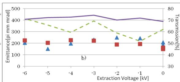
Figure 4: Squares are for x emittance measured by emittance monitor installed just after the FC3 and triangles are for y emittances. The dashed line shows the calculated emittance at the baffle slit the end of extraction system by IGUN code. The beam transmission between FC1 and FC3 is shown by solid line
