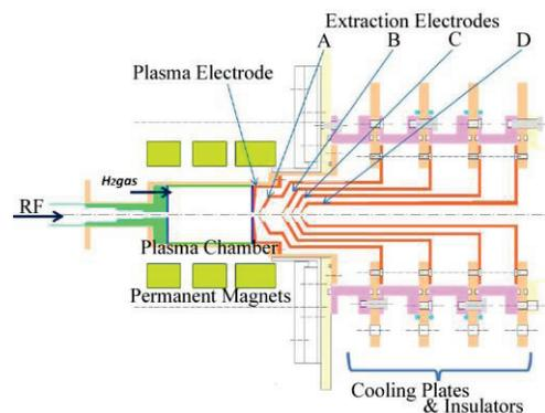
Figure 5: Schematic view of 2.45 GHz HIP-ECR. Extraction electrodes are connected to cooling plates separated by insulators.
