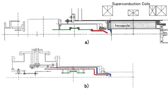
Figure 2: The schematic views of extraction system before modified in a) and after in b). In case of b) both positions of plasma and extraction electrode can be controlled from outside of vacuum chamber. New extraction electrode also can be applied to -20 kV. The baffle slit downstream of einzel lens is ground level.
