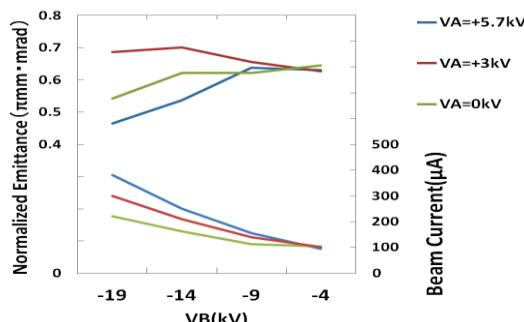
Figure 6: The proton beam production test with several conditions of applied extraction voltages. VA is the voltage of A-electrode shown in Figure 5. VB is for B-electrode. VC the C-electrode voltage is fixed to +4kV and VD is on ground. Upper lines show measured normalized emittances for each VA and VB. Lower lines show measured beam currents.
