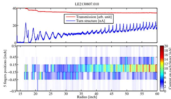
Figure 4: Measurement results from LE2 probe scan when injecting short bunches  $30^\circ$  off crest on the falling side of the rf wave. **Top:** the blue line shows beam current intercepted on the first 0.075 inch of the probe head; the red line shows the total current on the probe (arbitrary scale). **Bottom:** current read back on each of the five horizontal fingers.
