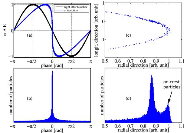
Figure 3: Macroparticle simulation of injection of short bunches: (a) longitudinal phase space right after the first harmonic buncher (black) and right before injection into the cyclotron (blue), in the absence of space charge; (b) phase distribution within the same beam before injection. The same particles, after crossing cyclotron acceleration gap, are shown in ‘top view’ (c), and in radial projection (d).
