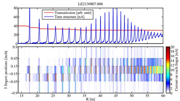
Figure 5: LE2 probe scan showing short bunches injected  $10^\circ$  off crest (falling side of the rf wave). (See caption of Fig. 4 for plot details.)
