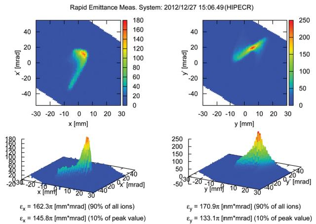
Figure 6: Result of analysis; phase space distributions and emittances in horizontal and vertical planes. 15 keV proton beam from 2.45 GHz ECR-IS.  $\epsilon_x \sim 160 \pi$  mm mrad,  $\epsilon_y \sim 170 \pi$  mm mrad
