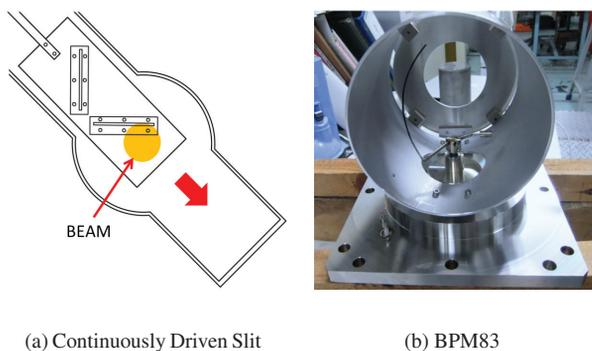
Figure 3: (a) Schematic diagram of continuously moving slit. (b) Photograph of BPM83 the beam profile monitor.
