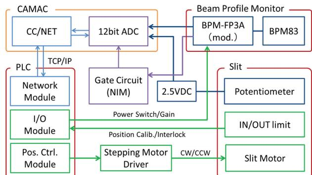
Figure 4: Control and data acquisition system.
