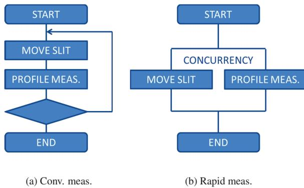
Figure 2: (a) Control sequence of conventional emittance measurement system. (b) Concept of rapid measurement by concurrency control.
