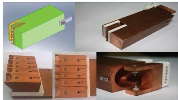
Figure 2: Structure of radial probe target tip 1.
