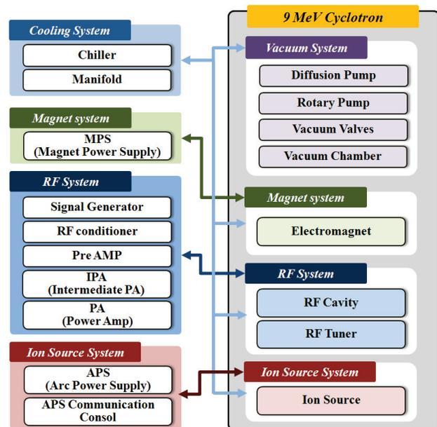
Figure 1: Configuration of 9 MeV cyclotron.
