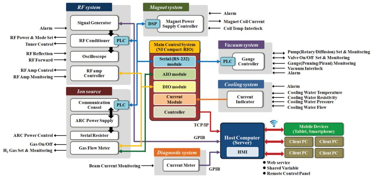
Figure 2: Architecture of 9 MeV cyclotron control system.
