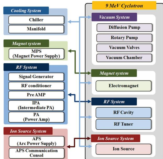
Figure 1: Configuration of 9 MeV cyclotron.
