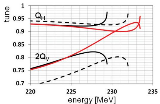
Figure 5: Tune functions. Red full line= measured with slightly horizontally displaced coil, black full line= measured with horizontally centered coil, black dashed line = design tune functions.
