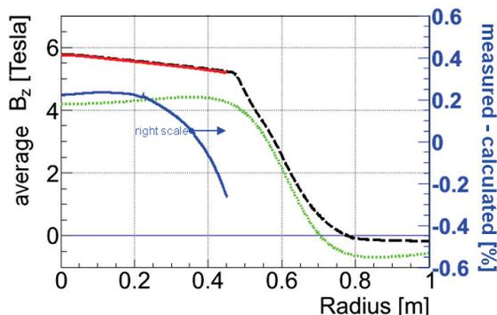
Figure 3 : Average field in the S2C2. Red full line= measured, black dashed line= calculated with OPERA3D, green dotted line= calculated pure coil field, blue full line (right scale)= deviation between measured and calculated average field.
