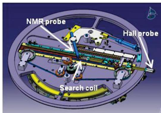
Figure 1: Layout of the mapping wheel.
