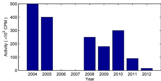
Figure 5: The cyclotron tank contamination level surveyed near the 1A foil position over the last several years (where the year 2006 and 2007's data were missing). It has been reduced by a factor of 5 to 10 in 2012.
