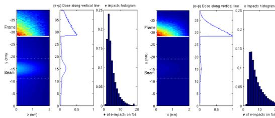
Figure 2: Results of simulation made with 5 (Left) and 1 mg/cm<sup>2</sup> (Right) foils, showing contours of energy deposit, distribution of energy deposit along  $y$ , and a histogram of number of electron impacts.
