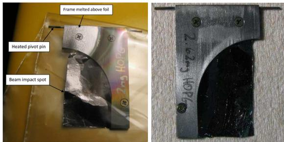
Figure 4: Left: The 3rd generation assembly, where the frame remained SS but had a larger radius. This was marginally successful but the frame still suffered some damage. Right: A used 4th generation foil/frame assembly which had accumulated about 176 mA-hr when it was removed in February, 2012. There was no visible damage to the foil or the Tantalum frame.
