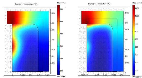
Figure 3: The foil (PG) and frame (SS) temperature distribution, calculated with 5 (Left) and 1 mg/cm<sup>2</sup> (Right) thicknesses. The darkest red is 1100°C.
