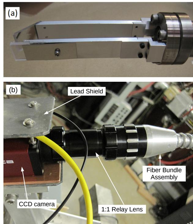
Figure 2: The two main components of the system: (a) Scanner Head with a steel mesh around the crystal for its charge neutralization. The mesh also provides mechanical support in case the crystal breaks. (b) The camera first connects to a relay lens and then to the SCHOTT Fiber Bundle; all connectors are C-mount.
