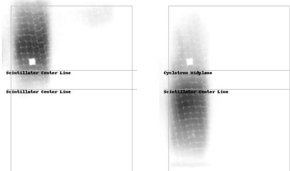
(a) Trim coil 1 in balanced mode (Top and bottom coil each run 356 A).
