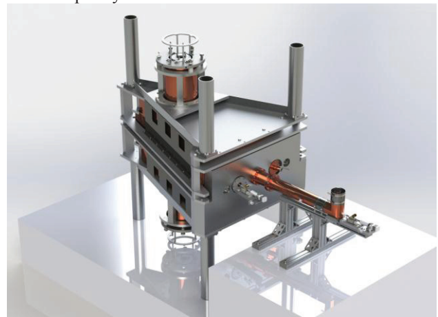
Figure 6: Resonator cold test set-up.
