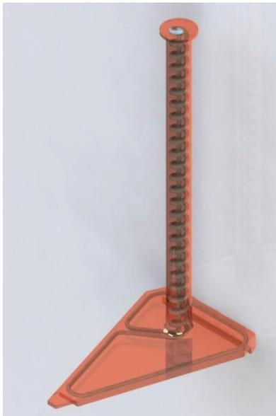
Figure 2: Geometry of cooling line second design.
