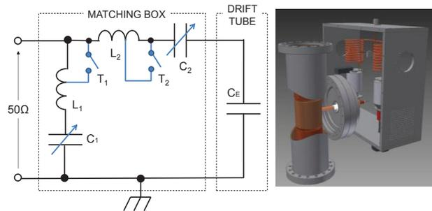
Figure 6: Matching-tuning box and drift tube.
