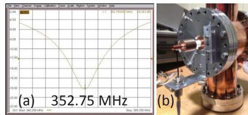
Figure 5: (a) Self-resonance, (b) N-type adaptor.
