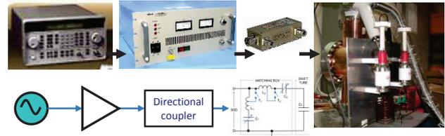
Figure 9: Test bench of the axial buncher at LNS.
