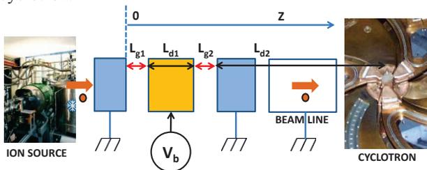
Figure 1: Basic structure of the axial buncher.
