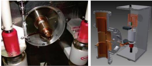
Figure 7: Direct connection between drift-tube and matching box.
