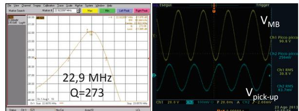
Figure 11: Q-factor, drift tube and pick-up voltages.
