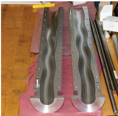
Figure 5: Photograph of the “snake” converter built.
