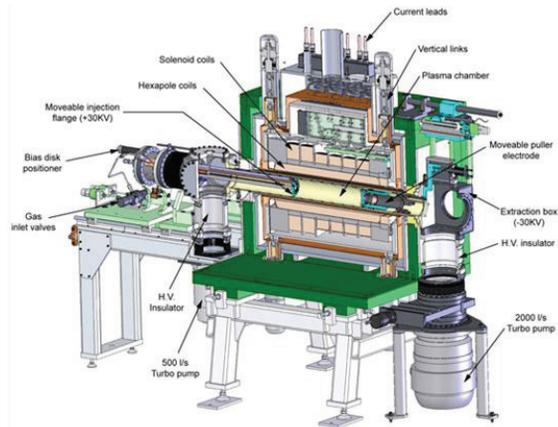
Figure 4: Sectional picture of SuSI source at NSCL.
