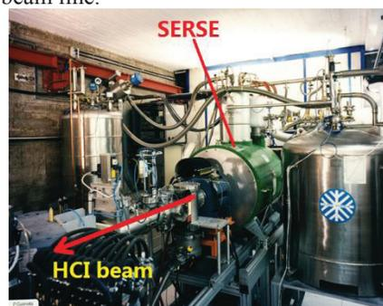
Figure 2: SERSE source installed to injector beam line.
