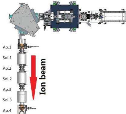
Figure 5: SuSI ion source and the collimation line.
