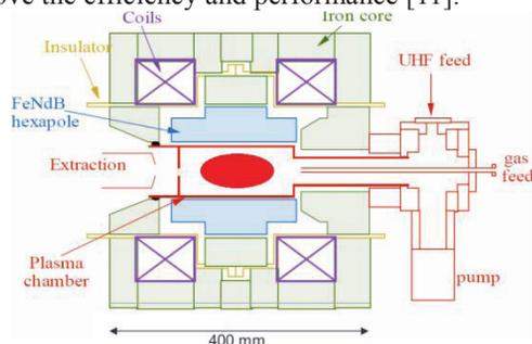
Figure 1: Schematic plot of ECR4 ion source.
