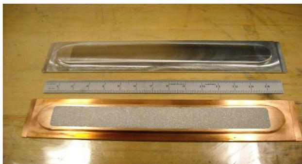
Figure 7: Top –  $^{209}\text{Bi}$  target on aluminum backing used in the production of  $\text{At-211}$ , Bottom –  $^{116}\text{Cd}$  target on copper backing used in the production of  $\text{Sn-117m}$ .
