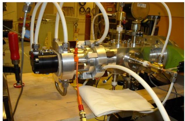
Figure 4: BruceTech liquid target module attached to the vault research beam line.
