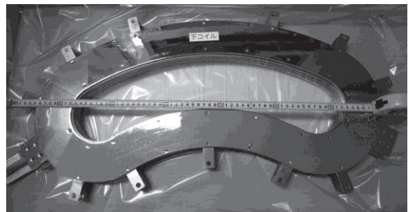
Figure1: Lower coil of the dipole magnet.
