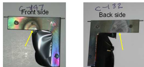
Figure 1: Used foils showing the signs of overheated frame and cracked and warped foil.
