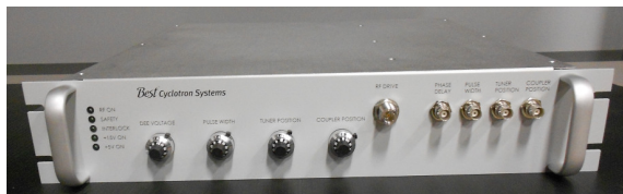
Figure 1: The front panel of the LLRF module showing status lights, local control potentiometers and RF I/O.
