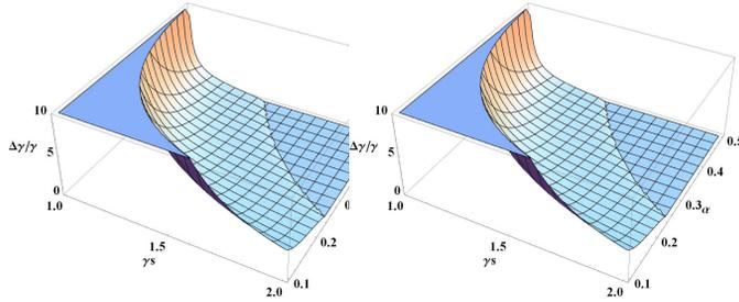
Figure 4: Normalized range (left) and required voltage (right) as function of  $\alpha, \gamma_{s1}$ . Range of  $\alpha = [0.1, 0.5]$ .
