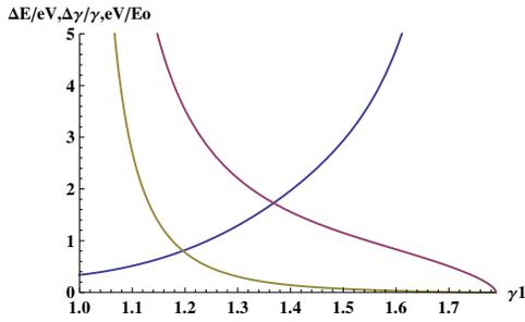
Figure 3: Range per volt ( $\Delta E/eV_0$ )/10 (blue), total range  $\Delta E/E_t$  (red), and minimum voltage  $eV_0/E_0$  (yellow).
