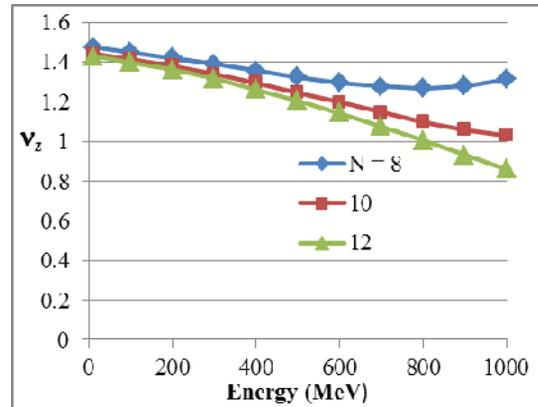
Figure 7: Variation of the vertical tune  $\nu_z$  with energy for  $H_1/B_c = 2$ ,  $H_2/B_c = 0.4$ ,  $h = 0.5$ , and various values of  $N$ .
