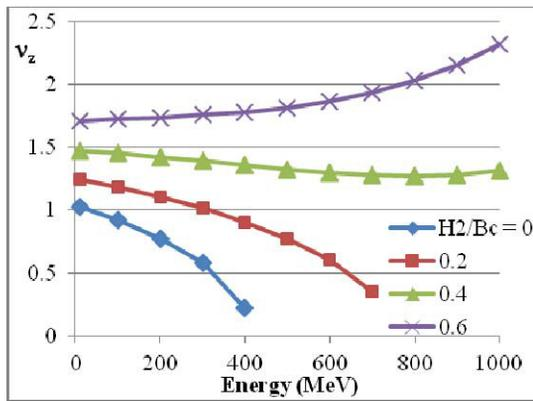
Figure 4: Variation of the vertical tune  $\nu_z$  with energy for  $H_1/B_c = 2$ ,  $h = 0.5$ ,  $N = 8$ , and various values of  $H_2/B_c$ .
