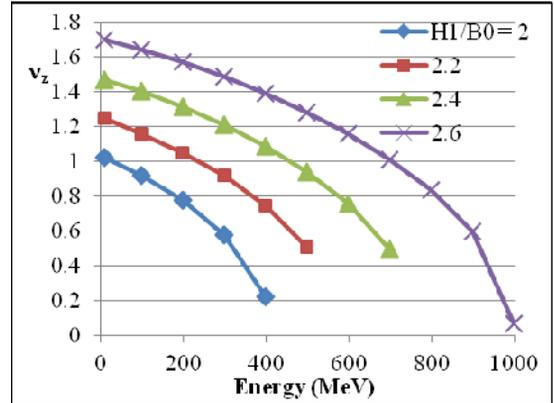
Figure 3: Variation of the vertical tune  $\nu_z$  with energy for  $H_2 = 0$ ,  $h = 0.5$ ,  $N = 8$ , and various values of  $H_1/B_c$ .
