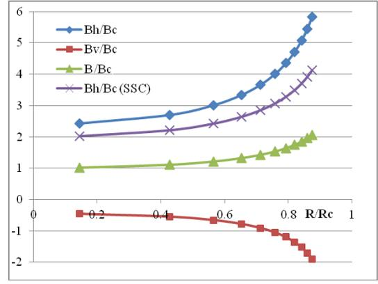
Figure 2: Field profiles for  $N = 8$ ,  $h = 0.5$ ,  $H_1 = 2B_c$ ,  $H_2 = 0.4B_c$ .
