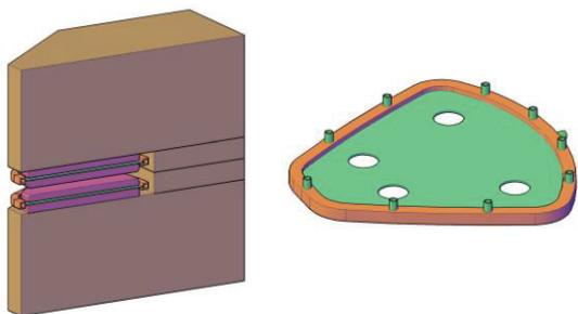
Figure 3: Half-cut model of sector magnet and support structure of main coil.
