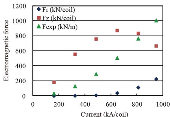
Figure 4: Electromagnetic force acting on the main coil as calculated by Opera-3d [3].  $F_r$  indicates a radial force from the cyclotron center to the outside. The vertical force  $F_z$  works in the upward direction for the upper coil.  $F_{exp}$  indicates the expanding force of the coils per unit length.
