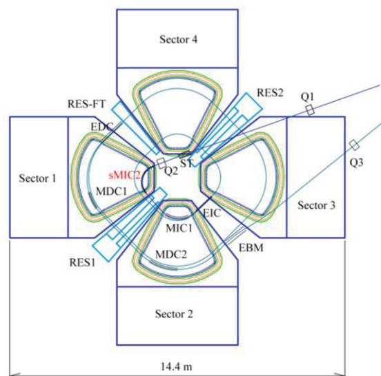
Figure 2: Plan view of new superconducting ring cyclotron.
