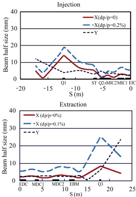
Figure 5: Beam envelope along the injection and extraction orbit. The blue line indicates the envelope for the beams with momentum dispersion.
