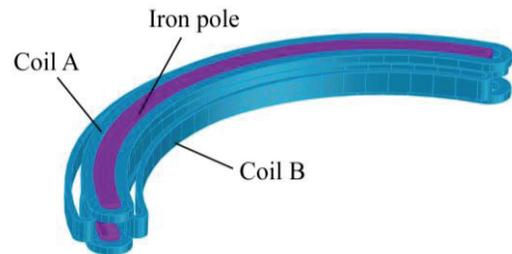
Figure 6: Superconducting magnetic channel sMIC2.
