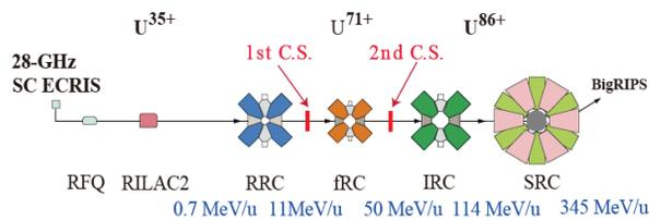
Figure 1: Existing acceleration system for U beam.
