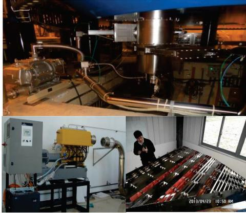
Figure 6: The installed dry pump and cryopumps (upper) and the cryopanel system (lower).
