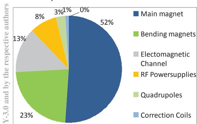
Figure 3: Energy consumption distribution for various parameters.
