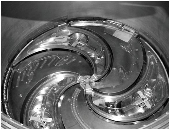
Figure 1: View of the median plane of the LNS Superconducting Cyclotron.
