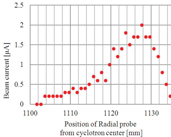
Figure 5: Beam profile by radial probe (30 MeV protons).
