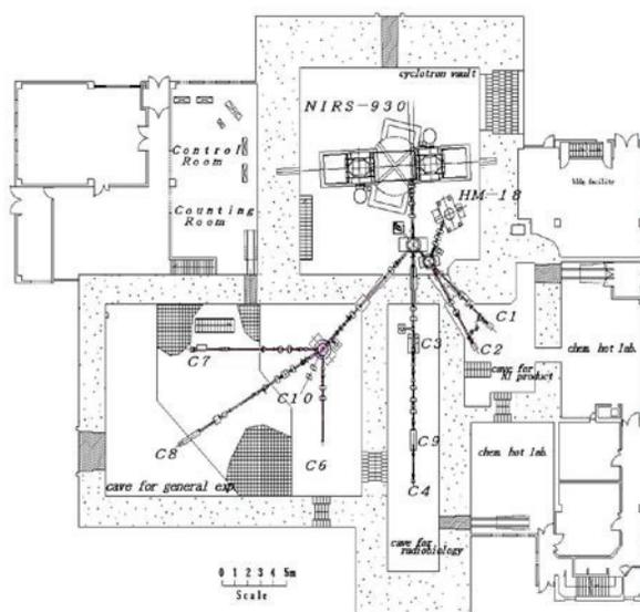
Figure 1: Layout of NIRS cyclotron facility.
