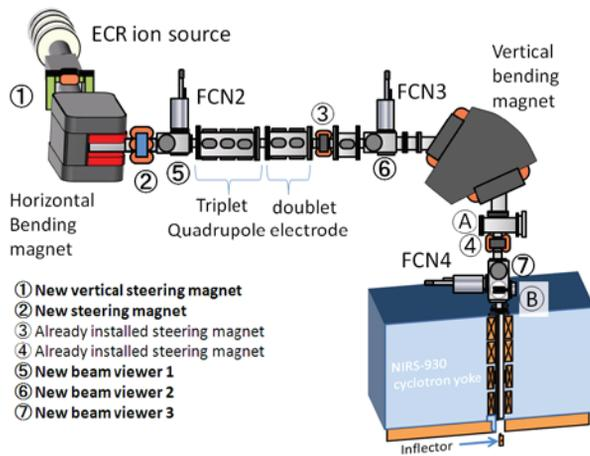
Figure 3: Layout of injection line for NIRS-930.
