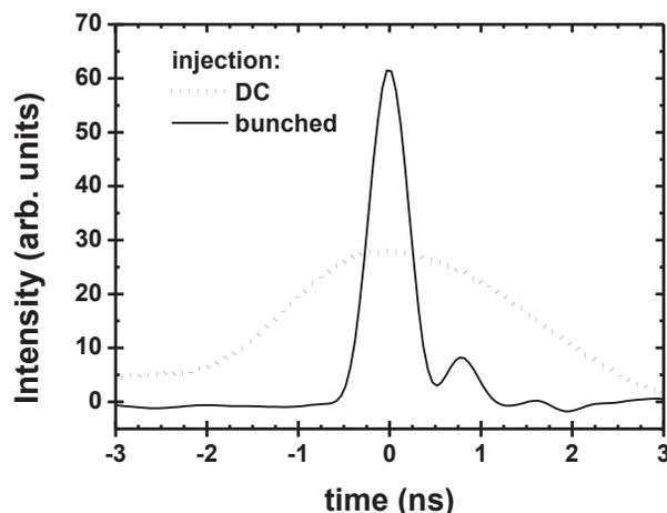
Figure 3: Pulses of the extracted 68 MeV proton beam measured with the coax-cup. The injected beam was a DC beam (dotted line) or a bunched beam (solid line). The second small peak visible is due to reflections.
