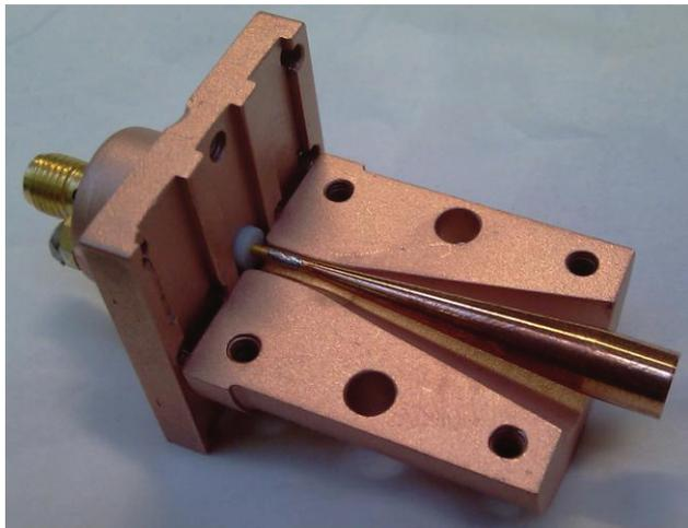
Figure 2: The open coax-cup without the acrylic glass in front (dielectric and support) and without shielding.
