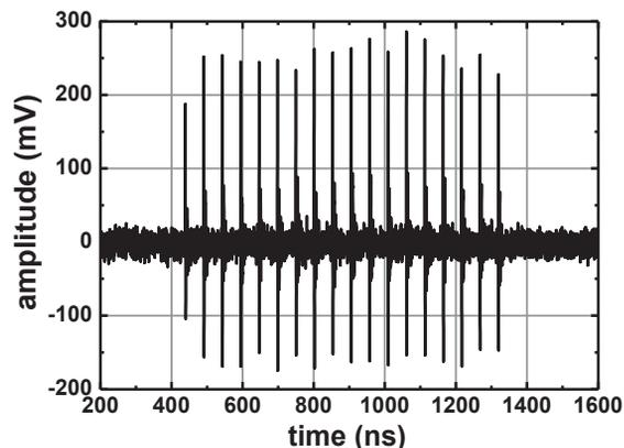
Figure 4: 1  $\mu$ s pulse packet of 68 MeV protons, measured with the pick-up. This time structure was used for the creation of pulsed neutron fields for dosimeter tests.
