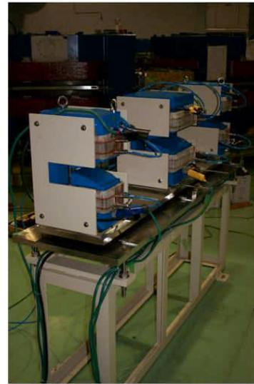
Figure 3: Picture of the straight scaling FFAG magnets prototype.
