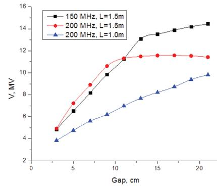
Figure 3: Maximum voltage gain as a function of gap width.
