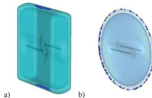
Figure 4: Areas of secondary particles growth in rectangular (a) and elliptical (b) cavities.
