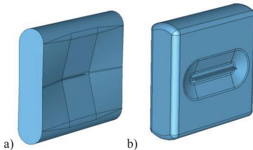
Figure 2: Rectangular cavity shapes before (a) and after (b) optimization.
