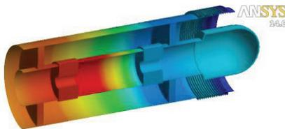
Figure 5: Temperature map of 100kW electric RF power coupler operating at cavity resonance (red 356K, blue 2K).
