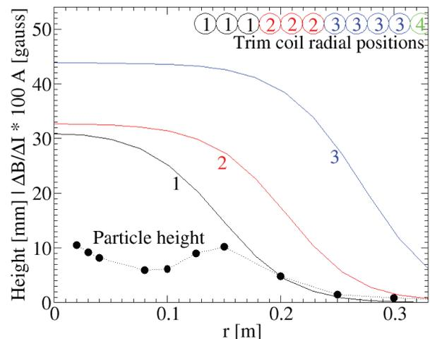
Figure 1: Equilibrium orbit heights for particle tracked through modelled magnetic fields are plotted as a function of radius with dots and a dashed line to guide the eye. The inner trim coil turns' radial positions are indicated at the top of the plot and the measured change in field per 100 A of current is plotted with the solid curves.
