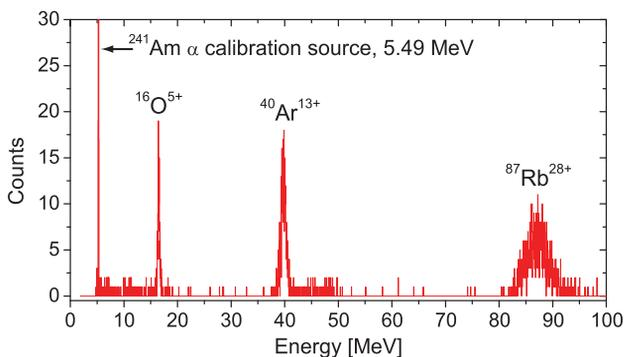
Figure 4: Measured energy spectrum of reaccelerated stable and long-lived isotopic beams.
