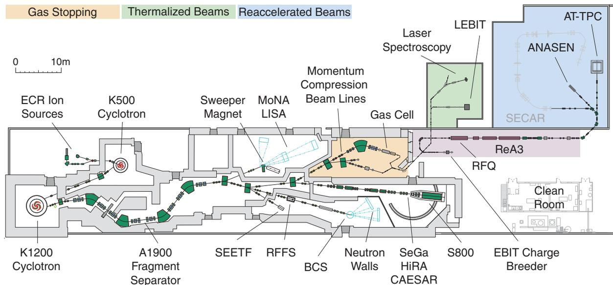
Figure 1: Facility layout of the National Superconducting Cyclotron Laboratory with the Coupled Cyclotron Facility and the newly commissioned gas stopping area and reaccelerated radioactive ion beam capabilities.
