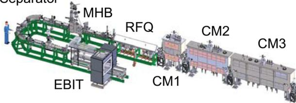
Figure 3: Overview of the ReA reaccelerator facility with EBIT charge breeder, Q/A mass separator, multi harmonic buncher (MHB), RFQ, beta=0.041 cryomodules (CM1 and CM2), and beta=0.085 cryomodule (CM3).
