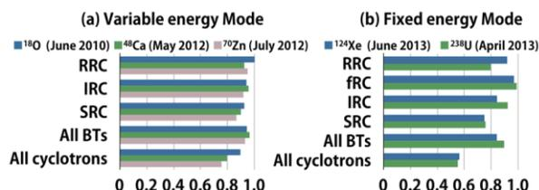
Figure 7: Transmission efficiency of the RIBF cyclotron cascade. BT means the beam transport line.
