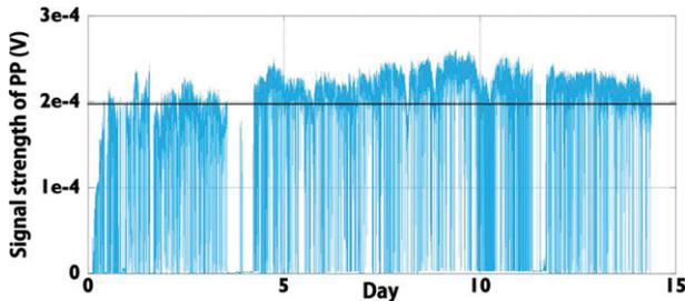
Figure 8: Stability of the beam bunch signal after the SRC for the 345 MeV/nucleon  $^{124}\text{Xe}$  beam recorded from 17 June to 1 July 2013.
