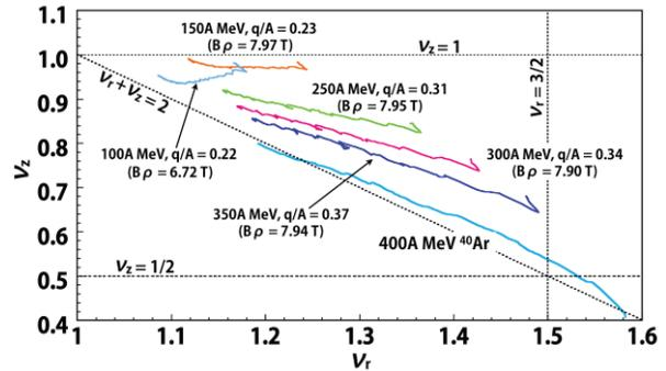
Figure 9: Tune diagram of the SRC. The difference in tune behavior in the extraction region between  $^{40}\text{Ar}$  and the others comes from the different optimization procedures used to generate isochronous magnetic fields. Back bending can be removed by changing the combination of excitation currents of the SC and NC trim coils.
