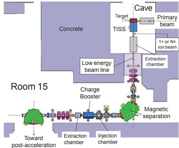
Figure 5: Schematic of the SPIRAL1 upgrade.
