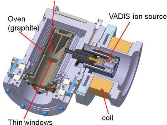
Figure 6: TISS made by association of a graphite target with a VADIS FEBIAD ion source.
