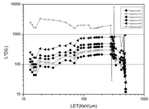
Figure 2: The distributions absorbed doses for various depths in CR-39 as  $L \cdot D(L)$  for a primary proton energy of 220 MeV.
