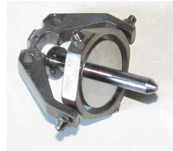
Compass with gimbal suspension
