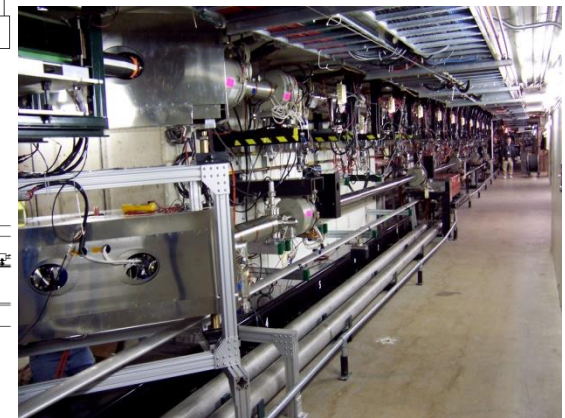
The Pelletron and beam “supply” and “transfer” lines
