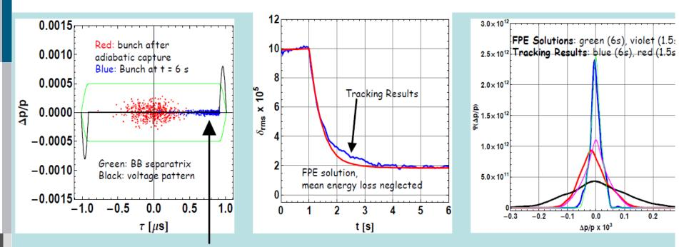
Strong bunching: bunch length  $\approx$  400 ns Beam no longer quasi DC as at 740 MeV/u with TOF cooling
