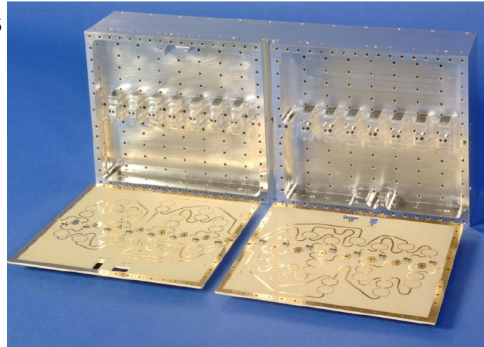
milled module body with combiner board
