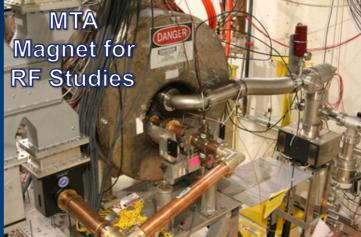
Operation of RF cavities in high magnetic fields is a necessary element for muon cooling
