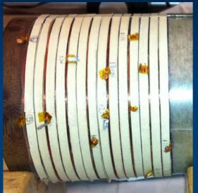
BSCCO-2212 Cable -Transport measurements show that FNAL cable attains 105%  $J_c$  of that of the single-strand
