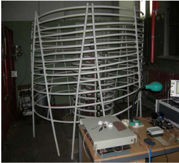
Fig.3 HV generator prototype U=300\text{ kV} , I=1\text{ mA}
