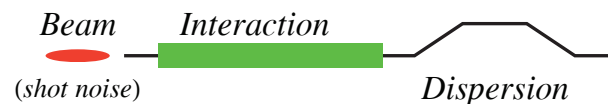
Figure 1: Schematic of noise suppression system. A beam with shot noise is injected into an interaction region of length L , followed by a dispersion region with a proper value of R_{56} .
